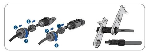
**Step 4**: Ensure that the cable is correctly positioned.
