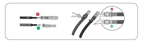
**Step 3:** Lead the cable through cable gland, and insert into the insulator until it snaps into place. Gently pull the cable backward to ensure firm connection. Tighten the cable gland and the insulator (Torque 2.5-3Nm).
