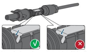
Release the clamping bracket. To do so, insert a screwdriver (blade width: 3.5 mm) into the clamping bracket and pry the clamping bracket open.
