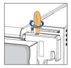
Step 2: Lead the sling through the two lifting rings and fasten the tie-down strap.
