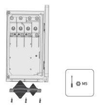
**Step 5:** Cut the appropriate hole in the tower guard coil according to the selected AC wire outer diameter specification.
