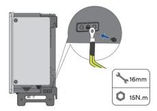
**Step 3**: Apply paint to the grounding terminal to ensure corrosion resistance.
