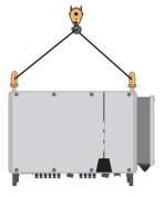
Step 4: Remove the lifting ring.
