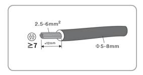
**Step 2:** Assemble the cable ends with the crimping pliers.
