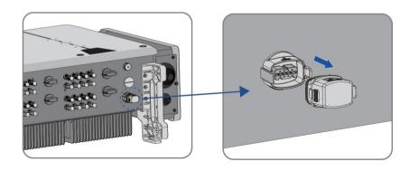
**Step 3**: Rotate the nut, take out the sealing ring, take out the plug , hold the locking structure, and take out the wiring terminal.
