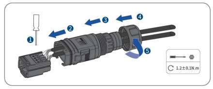
**Step 5** : Insert the completed RS485 communication terminal plug into the port, until it audibly snaps into place and confirm it is installed firmly.
