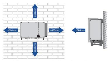
• In case of multiple inverters, reserve specific claerance between the inverters.
