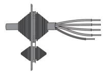
**Step 7:** Strip the protection layer and insulation layer by specific length, as described in the figure below.
