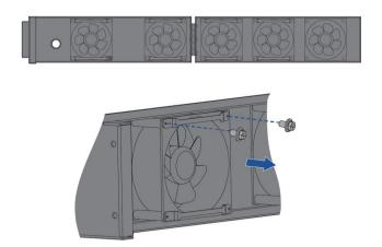
Step 5: Reinstall the fan back to the inverter in reverse order and restart the inverter.
