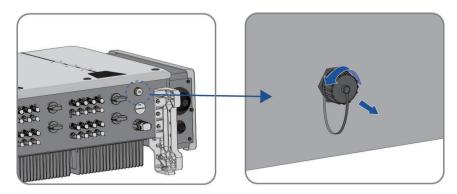
**Step 3**: Attach the WiFi modular to the connection port in place and tighten it into the port by hand with the nut in the modular. Make sure the modular is securely connected and the label on the modular can be seen.
