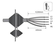
**Step 8**: Make the cable and crimp OT/DT terminal.
