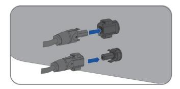
For unused DC connectors, push down the clamping bracket and push the swivel nut up to the thread. Insert the DC connectors with sealing plugs into the corresponding DC inputs on
